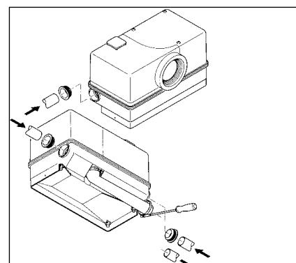
Put the plug-in seal(s) flush into the inlet sleeve(s). Then put the tube(s) up to the stop into the plug-in seal of the inlet sleeve. Push the pressure elbow with a strap over the pressure line and fix it.
