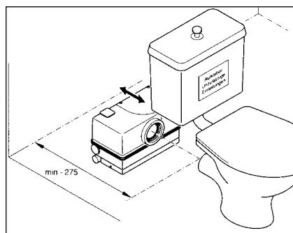
Put the pre-assembled WCfix 260 behind the toilet. Push the unit with the rubber collar DN 100 up to the stop (in the inlet of the tank) onto the outlet of the toilet. If necessary, moisten the rubber collar with soap water and level out the heights with the rubber bases of the unit with washers (not enclosed). Screw the sheet metal screws into the middle of the eyelet plugs.
