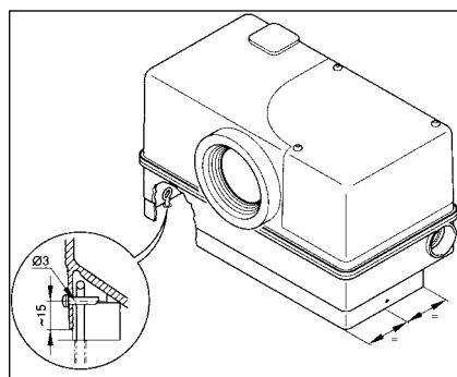
The WCfix 260 can be secured against torsion and floating by using eyelet bolts, dowels and sheet metal screws which are enclosed.
