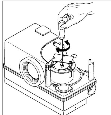
2. In case of any blockages of the unit: Insert a screwdriver through the hole in the Printed Circuit Board into the slotted pump shaft and turn it until the shaft is moving freely. Re-fit the cover and check the pump by a short test run.
