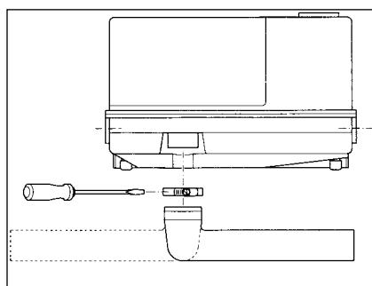
Push the pressure elbow onto the outlet of the unit, choose the direction and fix it with the strap. See to it that the pressure elbow is completely pushed onto the outlet, to secure a save installation of the strap.
