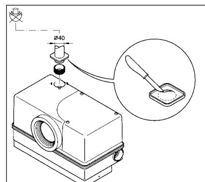
An uptake to the roof must be installed risingly. The connection of the line is
