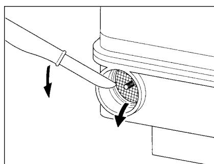
To connect a wash-basin, a shower and / or a bidet, remove the plug from the inlet. Pay attention to the installation notes concerning heights, falls and arrangement.
